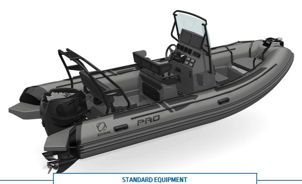
HULL & DECK: 2 aft cleats, 2 Fast flow bailers, Mooring bitt, 1 Bow D ring.
